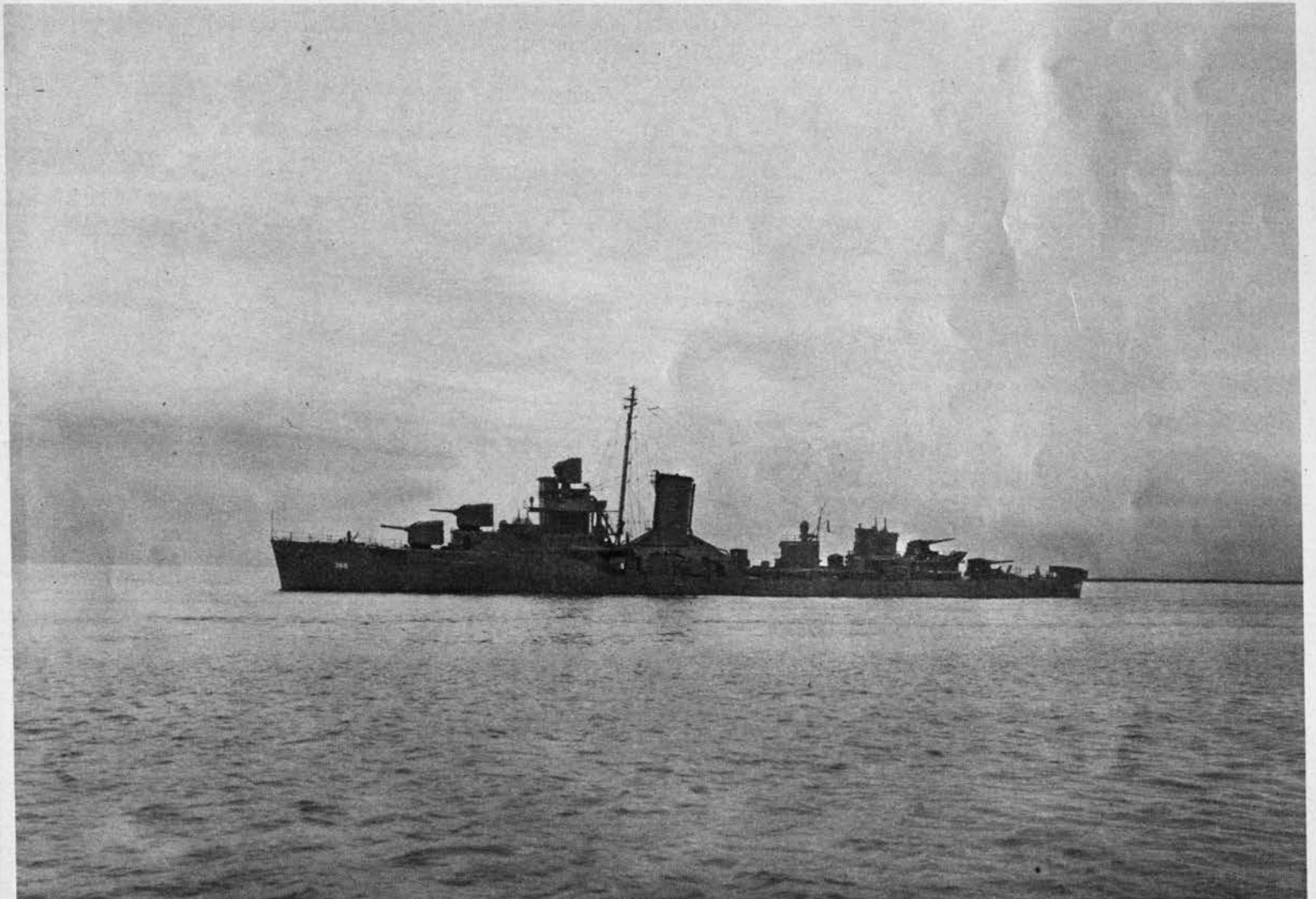
U.S.S. HELM shows split trunk which helps distinguish Bagley Class from the similar Gridley Class boats. U. S. fleet destroyers of the late
